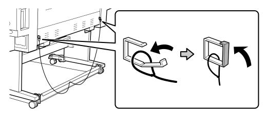
**8.** Attach the side loops on the basket to the front of the stand as shown.
