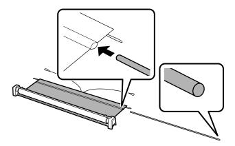
**4.** Fully extend the basket and pass it underneath the printer stand. Make sure the basket passes under the horizontal strut on the stand.
