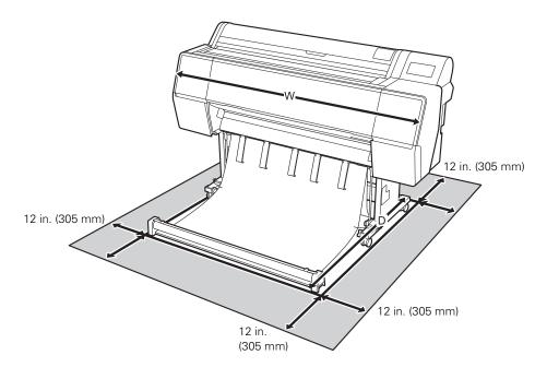
When choosing a place for the printer, choose a flat, stable location with adequate room for easy access and ventilation, near an outlet that meets the power requirements of the printer. Avoid locations subject to direct sunlight, excessive heat, moisture, or dust. Also avoid locations near potential sources of electromagnetic interference, such as loudspeakers, cordless phones, TVs, or air conditioners.
