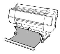
**16**. Attach the paper guides to the bottom of the printer. The SureColor P9500 Series has five guides, while the SureColor P7500 Series has two.
