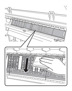
**4.** If paper particles have accumulated in the holes on the platen, use a toothpick or similar tool to push them through.
