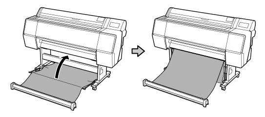
**14.** Attach the paper basket to the bolts on each side as shown.
