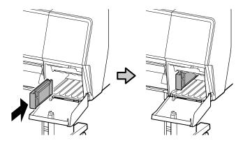
After installing all of the cartridges, close the ink covers. The printer begins charging the ink delivery system. Ink charging takes approximately 45 minutes.
