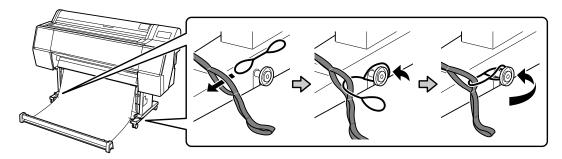
Note: You may not be able to eject paper correctly if the basket is too tight or is laying directly on the floor.
