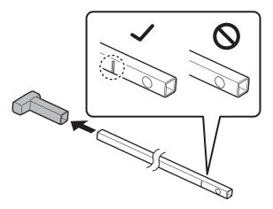
**10.** Insert the black plastic connectors onto the ends of the square rod.
