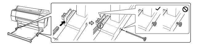
**13.** Lift the support rod into a vertical position.
