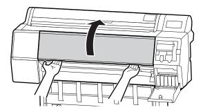
Wipe off any dust or dirt from the areas shown in gray. Wipe the platen from top to bottom, avoiding 3. the borderless pads.
