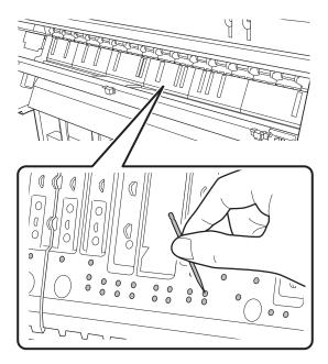
5. Using a cotton swab, clean any dust or dirt from around the borderless pads as shown below.
