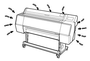
3. Open the roll paper cover and remove the tape and packing material.
