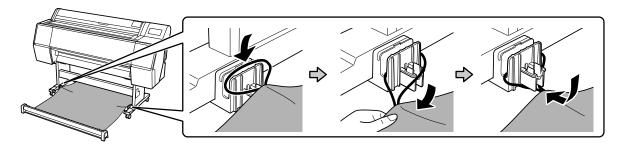
9. Insert the square rods into the ends of the black plastic connectors.
