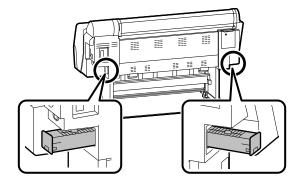
**Note:** The P7500 Series has one maintenance box, located on the right of the printer.
