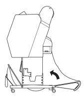
Raise the paper guides, then adjust the tabs and raise the front of the basket. Lower the paper guides.
