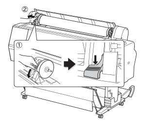
Roll the paper forward so that it rests on top of the printer.
