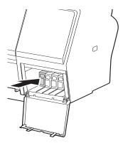
5. Remove the expended ink cartridge from the printer. Save your first set of expended cartridges so you can use them for transporting the printer, if necessary.
