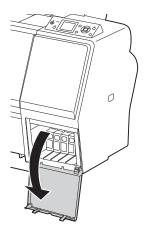
Press in the cartridge you want to replace. The cartridge pops out.
