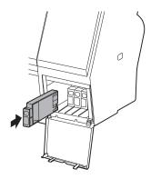
**Caution:** Do not remove and re-insert cartridges more often than necessary. Doing so can compromise the needle valve seal and allow air to enter the ink tubes, causing nozzle damage.
