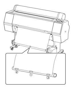
2. Press the ▼ button to feed the paper forward and create some slack.
