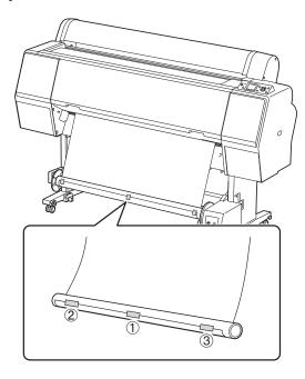
Press the ▼ button to feed the paper forward and create some slack.
