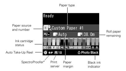
Note: The LCD screen of the SC-P7000/SC-P9000 is shown with the Violet (V) ink configuration. The ink cartridges shown will vary based on the printer model.
