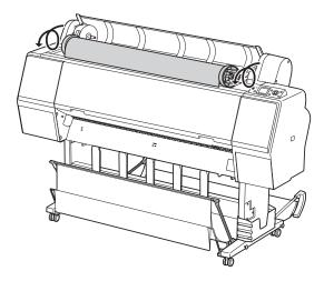
Pull up the tension levers, then remove the adapters from the paper roll.
