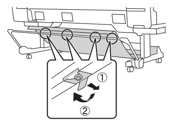
2. Loosely roll the basket cloth and insert the loops into the clamps on the bottom of the printer.
