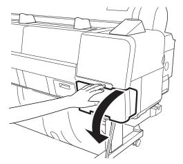
**3**. Insert a finger into the notch in the top of the cartridge and pull it straight out of the printer. Save your expended cartridges so you can use them for transporting the printer, if necessary.
