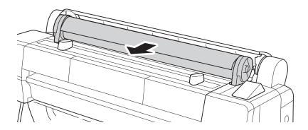
Release the tension levers on both adapters. 7.
