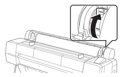
**6.** Lift the roll out of the printer and place it on top of the paper guides.
