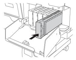
**Caution:** Do not remove and re-insert cartridges more often than necessary. Doing so can compromise the needle valve seal and allow air to enter the ink tubes, causing nozzle damage.
